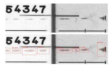
Measuring the  $V^2$ d is not easy or trivial. It is done through X-ray pictures (e.g. Figures 4 or 7). A grey scale value has to be defined to determine where the Shaped Charge jet diameter "ends". Experiments with different grey scales gave different diameters by almost a factor of two. Also the measuring of the jet velocity behind a steel barrier P is not trivial and can be a source of additional scattering - exacerbated by the squaring of the velocity.
