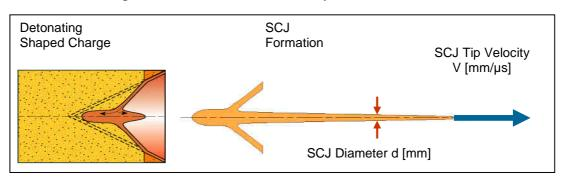
Figure 1: Determination of SCJ velocity V and SCJ diameter d
