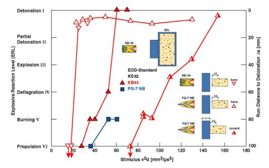
Figure 8: Item responses vs. V2d stimulus according to test configurations (MBDA TDW)
