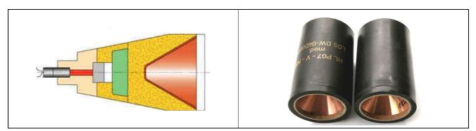
Figure 5: German PG-7 replica (75 mm diameter)
